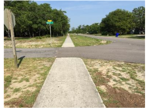
Existing Oak Island Drive sidewalk provides excellent east to west access for pedestrians, but should be widened to a minimum of 8' to account for joint use by cyclists. Image Source: HCP, Inc.
